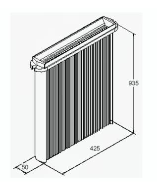
The R03 Venting Filter is provided with seven filter elements.
